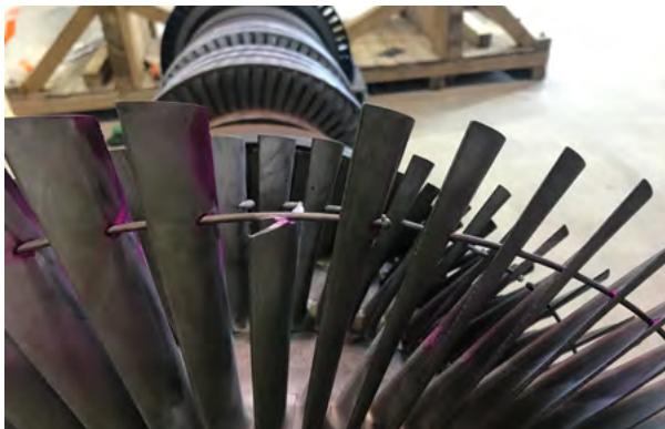
▲ A blade has been broken due to the turbine operating outside its designed vibrational environment
